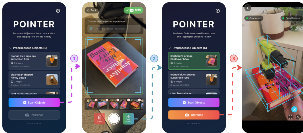
Fig. 1. The POINTER end-to-end workflow. (1) The user begins at the main inventory screen and initiates a scan. (2) During scanning, the user captures sparse, multi-view images of a novel object to generate semantic and geometric priors. (3) During inference, the system robustly estimates the real-time pose of a target object and anchors interactive digital content directly to it.
